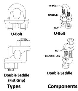
Figure 24 Wire Rope Clips
